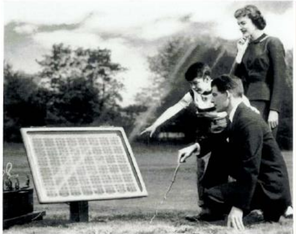
Something New Under the Sun. It's the Bell Solar Battery, made of thin discs of specially treated silicon, an ingredient of common sand. It converts the sun's rays directly into usable amounts of electricity. Simple and trouble-free. (The storage batteries beside the solar battery store up its electricity for night use.)
