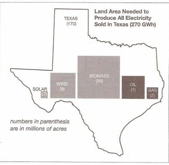
LAND AREA NEEDED FOR VARIOUS TEXAS ENERGY SOURCES Each square shows the land area needed by different energy resources to produce enough electricity for the entire state of Texas. Oil wells and wind turbines produce about the same amount of energy per unit of land area.
