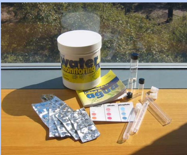
Typical low-cost water quality monitoring kits test for dissolved oxygen, nitrates, phosphates, fecal coliform bacteria, pH, temperature, and turbidity. Photo by D. Ruez, 2005.
